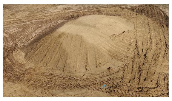
Dense Point Cloud with the Surface for Volume Calculation
